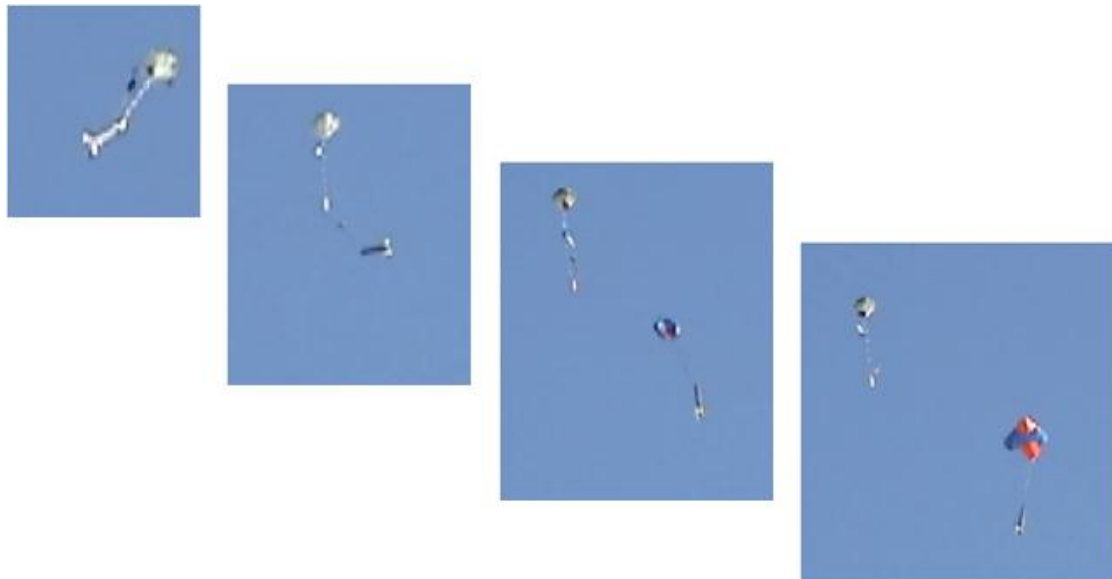
Figure 14 Recovery Package Consisting of Dual Deployment via Tender Descender
