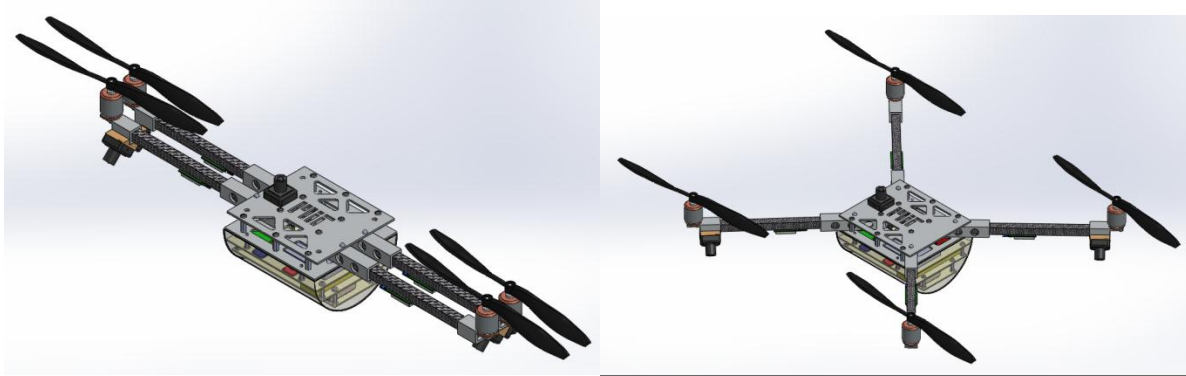
Figure 33 The Folded and Unfolded configurations of the quadrotor arms
