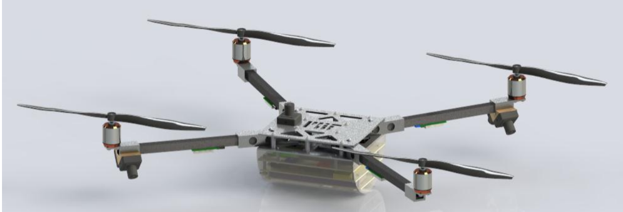
Figure 28 The Current Design of Quadrotor and Science Sensor Suite Configuration
